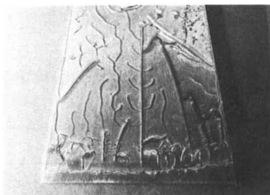
FIGURE 4 Fracture surface of silicone rubber layer, 1 mm thick. The end width of the steel plate is 100 mm.
